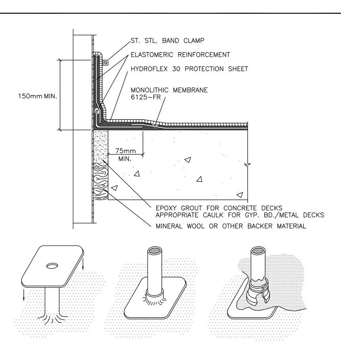
NOTES: PENETRATION MUST BE PROPERLY SECURED TO STRUCTURE TO PREVENT VERTICAL OR LATERAL MOVEMENT.
