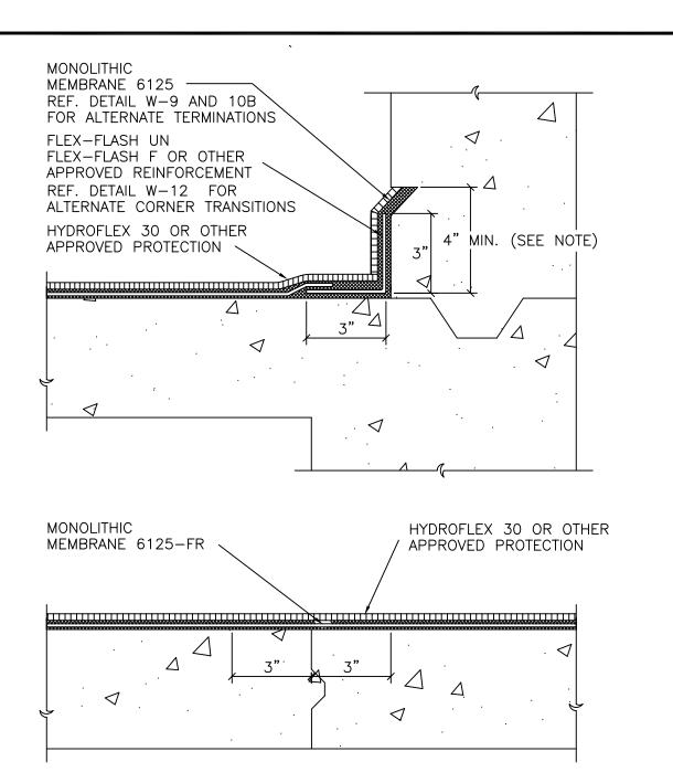
NOTES: IN COVERED/BURIED CONDITIONS, MM 6125 IS EXTENDED AS CONTINUOUS FLASHING AS HIGH AS POSSIBLE. FLASHING MUST BE TERMINATED NO LESS THAN 4" ABOVE SUBSTRATE.
