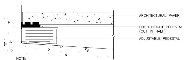
AT TYPICAL TERMINATION POINTS, THE ADJUSTABLE PEDESTAL IS PLACED SUCH THAT 1/2 OF A FIXED HEIGHT PEDESTAL MAY BE BUTTED UP TO THE STRUCTURE (curb, wall, ect.)
