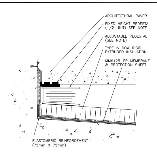
NOTES: TYPE IV DOW RIGID EXTRUDED INSULATION MUST BE 60 PSI (414 kPa) (COMPRESSIVE STRENGTH) BOARD MINIMUM.
