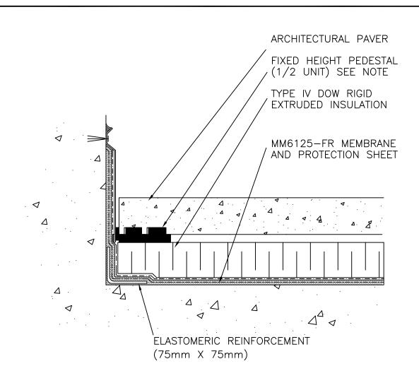
NOTES: TYPE IV DOW RIGID EXTRUDED INSULATION MUST BE 60 PSI (414 kPa) (COMPRESSIVE STRENGTH) BOARD MINIMUM.
