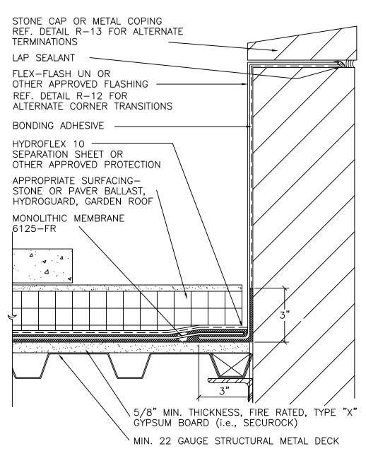
NOTES: ADEQUATE STRUCTURAL SUPPORTS AND THE NUMBER AND TYPE OF FASTENERS REQUIRED TO COMPLY WITH APPLICABLE CODES, SHOULD BE DETERMINED AND VERIFIED BY PROJECT ARCHITECT/ENGINEER.
