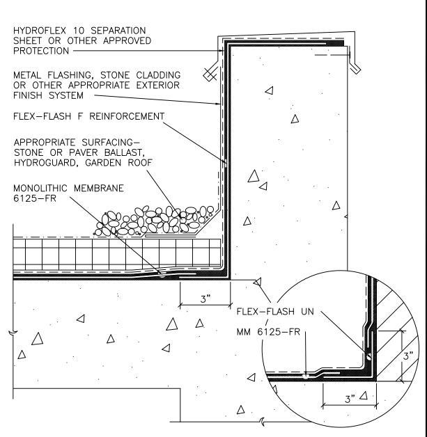
NOTES: MONOLITHIC MEMBRANE 6125 CAN BE USED TO FLASH PERIMETER PARAPET/ CURB DETAILS BUT MUST NOT BE LEFT EXPOSED.
