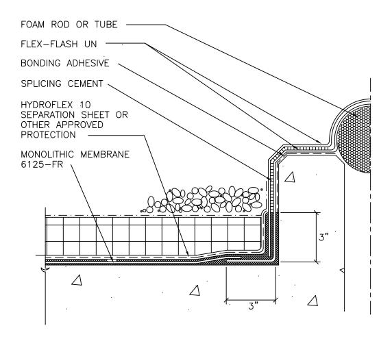
NOTES: TREATED WOOD BLOCKING, CONCRETE MASONRY UNITS, ETC., CAN BE SUBSTITUTED FOR P.I.P. CONCRETE CURB.
