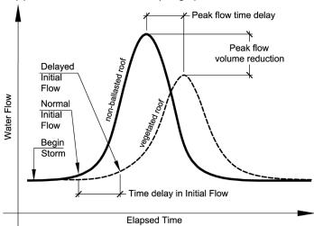
Civil engineers use hydrographs to predict the performance of stormwater BMPs. Comparing hydrographs from non-vegetated and vegetated roofs can determine the delay in the peak flow and the reduction of the peak volume.
