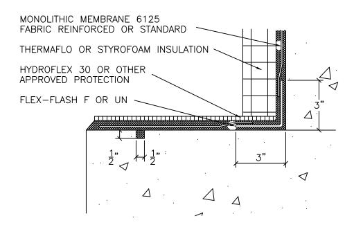
NOTES: WHEN FOUNDATION WALLS ARE CONSTRUCTED OF CONCRETE BLOCK (CMU), MM 6125 MUST BE INSTALLED IN FABRIC REINFORCED MEMBRANE ASSEMBLY.
