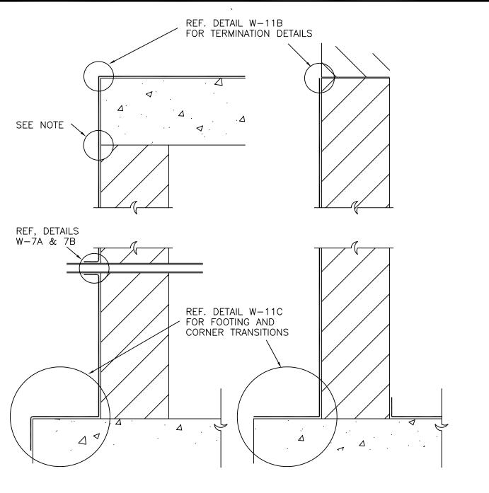
NOTES: WHEN FOUNDATION WALLS ARE CONSTRUCTED OF CONCRETE BLOCK (CMU), MM 6125 MUST BE INSTALLED IN FABRIC REINFORCED MEMBRANE ASSEMBLY.
