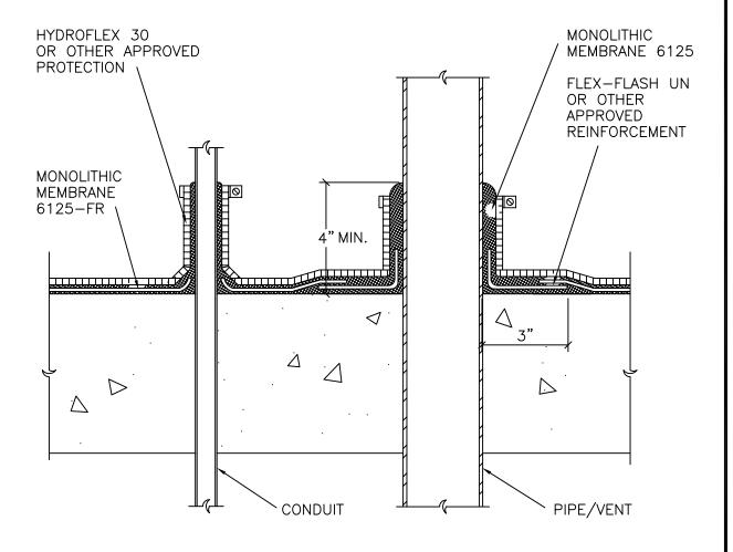
NOTES: SOME PIPE MATERIALS (PVC, COPPER, BRASS) MAY REQUIRE ROUGHENING/ SANDING, IN ADDITION TO PRIMING W/SURFACE CONDITIONER, FOR PROPER ADHESION OF MM 6125.
