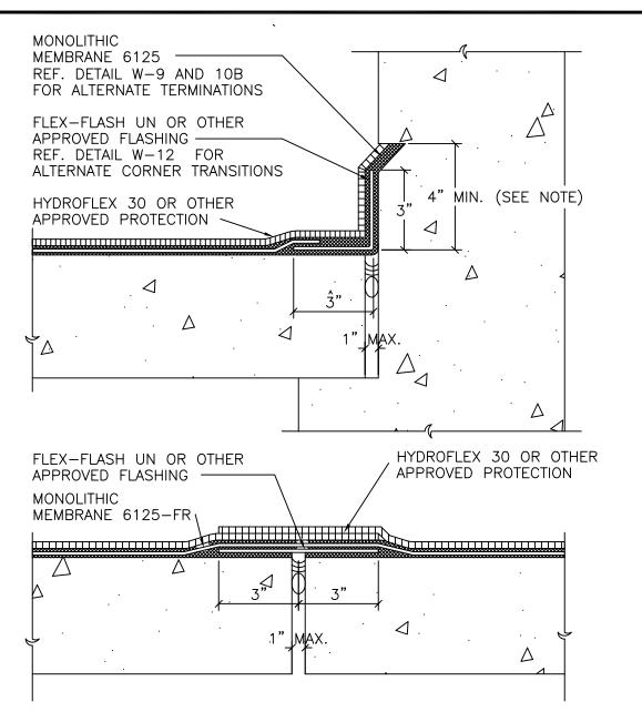
NOTES: DETAIL DESIGNED TO ACCOMMODATE MAX. 50% TOTAL MOVEMENT.
