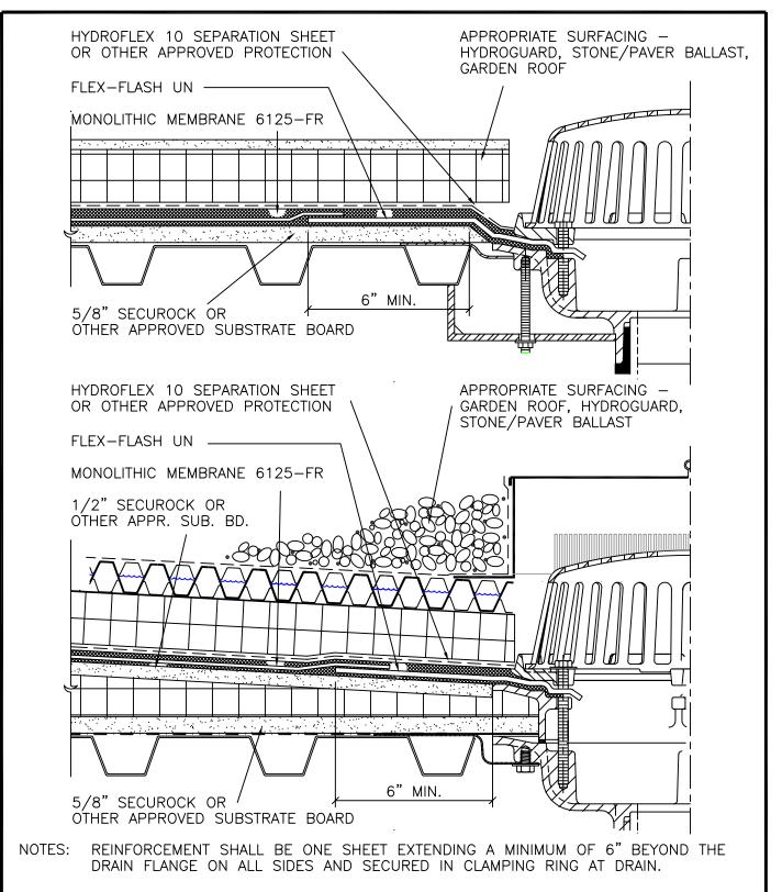
ALL DRAINS ARE REQUIRED TO HAVE FLASHING CLAMPING RING ASSEMBLIES. CONSULT SPECIFIC DRAIN MANUFACTURER FOR ADDL. ACCESSORIES (i.e., PERFORATED GRAVEL COLLARS, UNDERDECK CLAMPS FOR METAL DECKS, ETC.)
