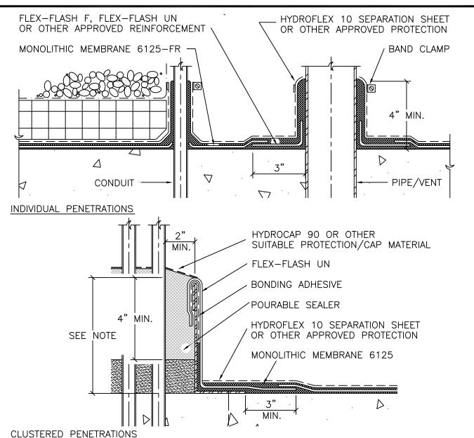
NOTES: TOP OF PITCH POCKET (TOTAL HEIGHT) SHOULD BE AT OR HIGHER THAN THE SURFACE OF THE BALLAST/TOPPING. MEMBRANE "FILL" MUST BE A MINIMUM OF 4" DEEP. EXCESS DEPTH MAY BE FILLED WITH A NON-SHRINK GROUT.
