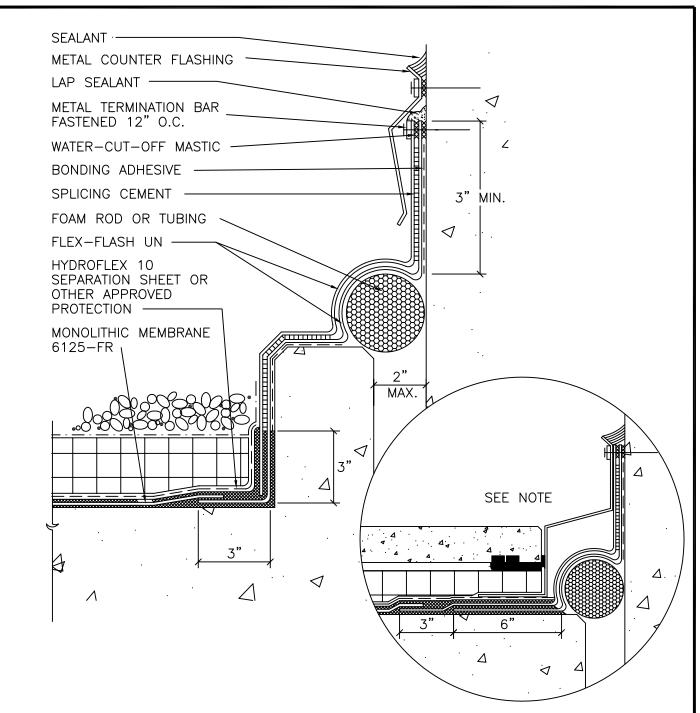
NOTES: TREATED WOOD BLOCKING, CONCRETE MASONRY UNITS, ETC., CAN BE SUBSTITUTED FOR P.I.P. CONCRETE CURB.
