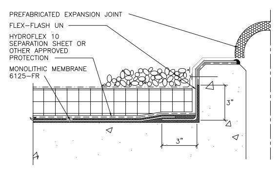
NOTES: TREATED WOOD BLOCKING, CONCRETE MASONRY UNITS, ETC. MAY BE SUBSTITUTED FOR P.I.P. CONCRETE CURB.
